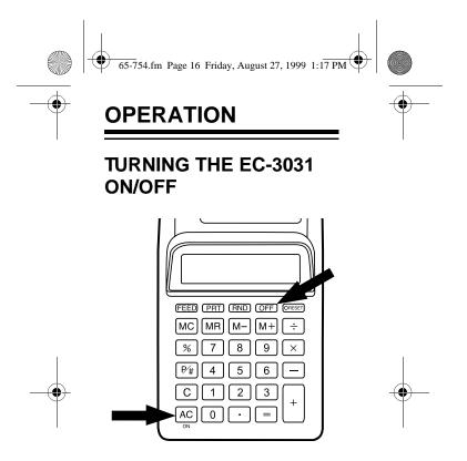
Press AC to turn on the EC-3031. Press OFF to turn it off.
